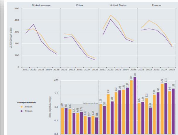
Figure 9.4 Turnkey BESS prices by market and duration, 2021-2025
